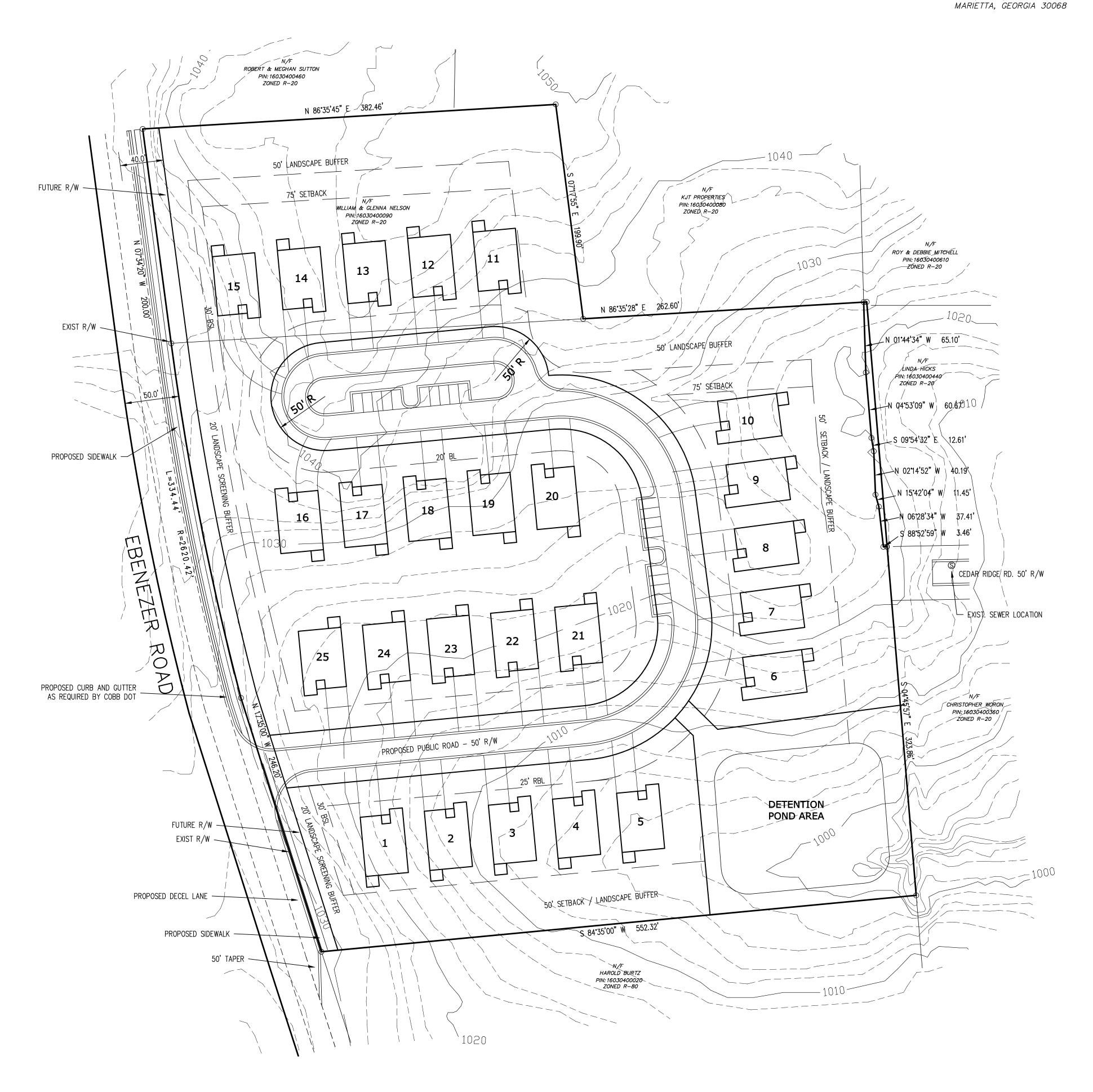
IF STATE WATERS ARE DISCOVERED TO EXIST ON THIS SITE A 25' BUFFER MEASURED FROM THE TOP OF BANK SHALL REMAIN UNDISTURBED AND SUBJECT TO ALL THE REGULATIONS GOVERNING STATE WATERS.
