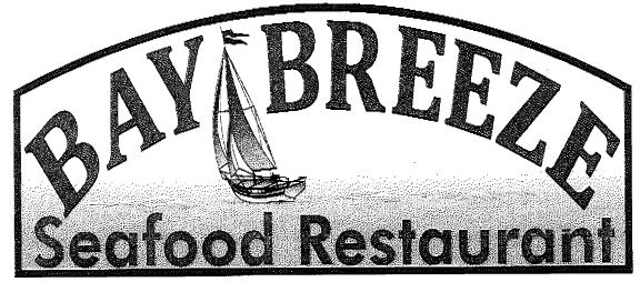
Double Sided: Non-illuminated cabinet with channel letters internally illuminated with exposed neon. Boat to be digital printed graphics applied to lighted logo box.
